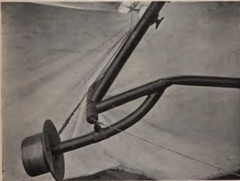
Fig. 80.—The outrigger wheel that gave out and caused an accident with the machine.
